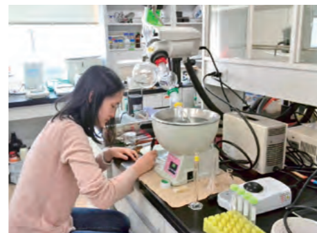
発酵茶中の機能性成分の解明。機能性成分を含む画分の濃縮を行っているところ Elucidation of bioactive compound in fermented tea - a picture of evaporation of fraction containing bioactive compound-
