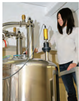
農産物中の生理活性成分の化学構造を解析する核磁気共鳴装置 (NMR) The nuclear magnetic resonance apparatus for identification of a bioactive compound in an agricultural produce
